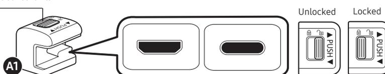
**A1** Stop and verify which USB port your phone corresponds to. For USB type-C move to the main setup for micro USB, complete A2-A3 before setup.
