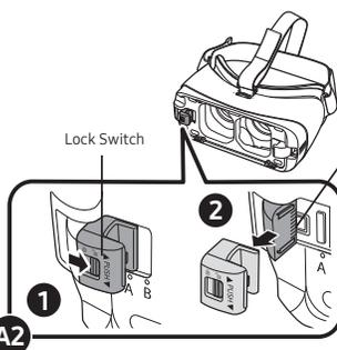
**A3** (1) Slide the Micro USB adapter into the connector base until firmly seated (2) slide left on adapter lock until you here a click. your Micro USB adapter is now in place. Proceed to Gear VR Setup Prompt.
